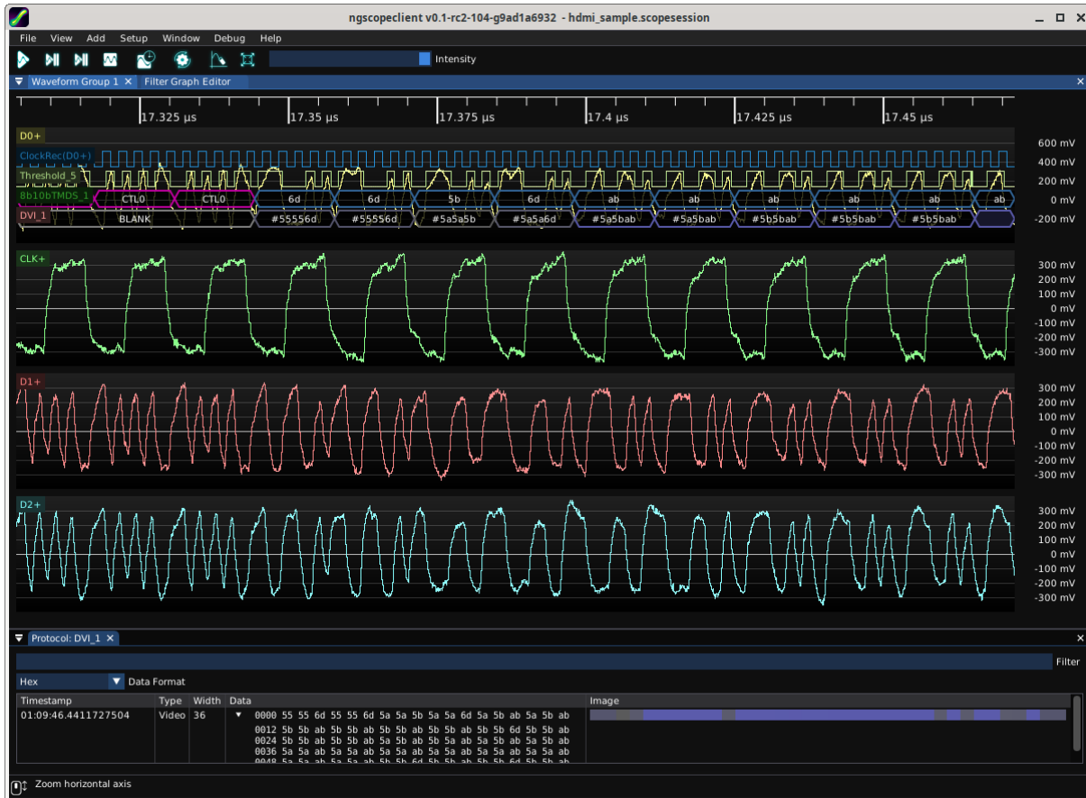
Figure 26.61: Example of decoding a DVI signal
