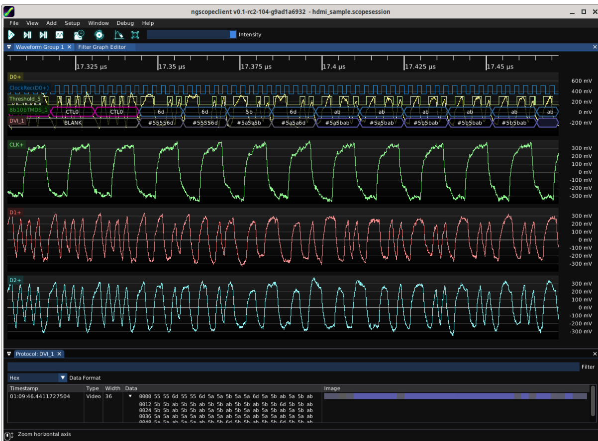
Figure 26.7: Example TMDS decode
