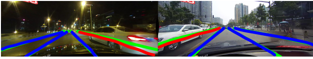
Figure 6: Evaluation based on IoU. Green lines denote ground truth, while blue and red lines denote TP and FP respectively.
