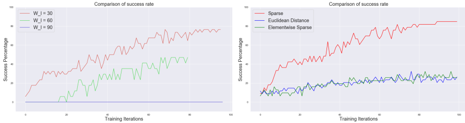
Figure 6: Left: Role of low level window size in RPL. As the window size increases, imitation learning and fine-tuning become less effective. Right: Role of fine-tuning reward function in RPL. We see that the sparse reward function is most effective once exploration is sufficiently directed.
