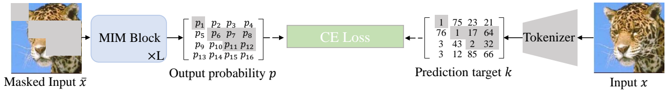
Figure 2: (a) Training pipeline of our Perceptual Codebook. (b) Apply PeCo in BERT-Like pretraining. Our PeCo provides a more semantic prediction target to the Mask Image Modeling Task.
