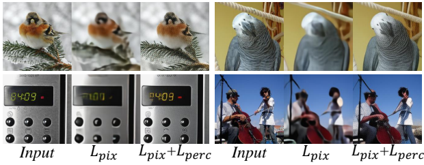
Figure 3: Image reconstruction with different losses. An example contains three images showing input (left), reconstructed image using pixel-wise loss (middle), and reconstructed image using pixel-wise and feature-wise losses (right). We can see that perceptually the right image appears more similar to the input compared with the middle image, although the middle image gets lower pixel-wise loss.
