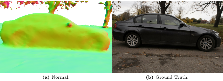
Fig. 13: Mesh Extracted by Neuralangelo [30]. The left figure illustrates the normals obtained by rendering the mesh extracted by Neuralangelo [30] from the corresponding viewpoints of the ground truth. While Neuralangelo [30] can reconstruct foreground objects well, it still struggles to accurately model background details.
