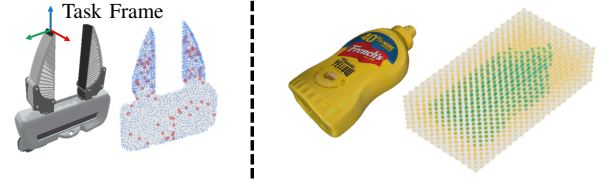
Fig. 3: Left: The gripper’s geometry is represented by a point cloud: 1000 points sampled on the surface (blue) and 50 inside the volume (red) of the mesh model. The task frame is defined at one fingertip. Right: The object (i.e., mustard bottle) is modeled by a signed distance field (SDF), where positive and negative values are visualized by yellow and green points respectively.
