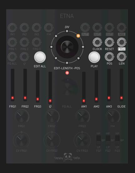
Etna can be synchronized with an external clock by connecting a signal to the CLOCK input jack. It will advance to the next stage with each pulse, allowing you to send trigger patterns to play the snapshots. By holding the encoder for 3 seconds, you can divide the clock rate to enable slower morphing through the snapshots. Sending triggers to the RESET input jack will return the PLAY LED to Snapshot 1.
