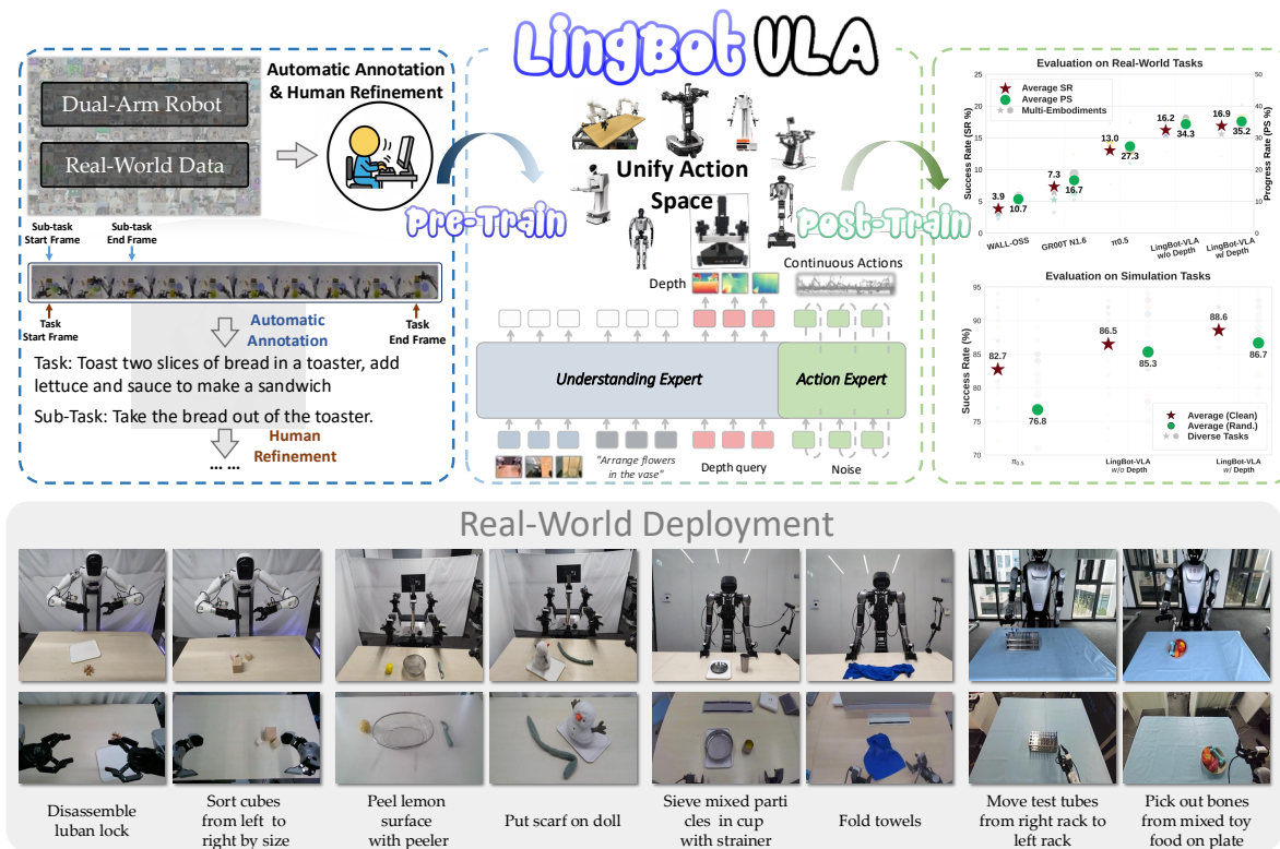
Figure 1. Overview of LingBot-VLA. We scale dual-arm robot data collected in the real world for pre-training. LingBot-VLA can be easily and efficiently transferred to downstream tasks. Moreover, we conduct a systematic assessment across three robotic embodiments, which demonstrates the clear superiority of our model.
