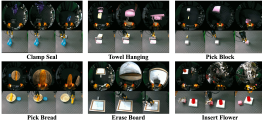
Figure 5: Real-world rollout of the data efficiency policy. Only fisheye camera input to the model.
