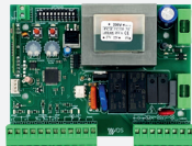
COD. E102/P E102 control board with bollard software + receiver
