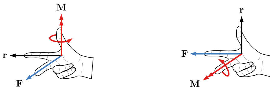
Figure 4.1.5 Three-finger right-hand rule for moments.
