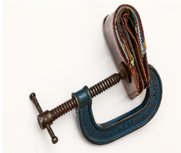
(b) A C-clamp screw rotates and translates through a fixed nut.
