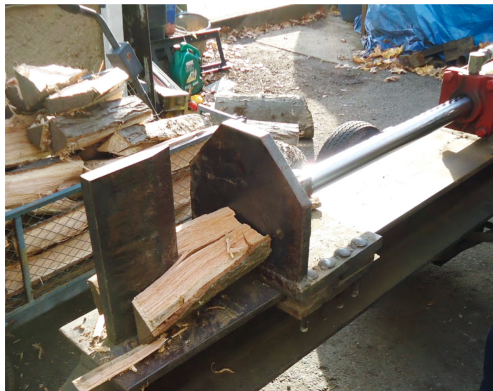
(a) A low friction wedge is used to split logs.
