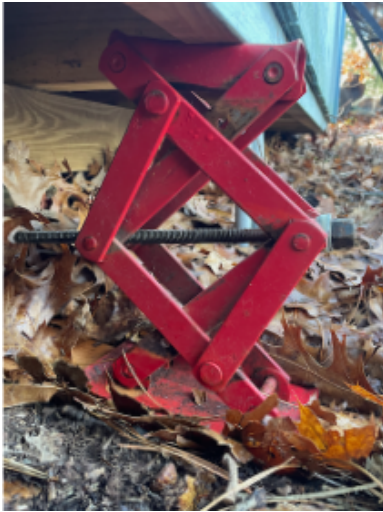
(a) A scissor jack uses fixed screw and a moving nut.
