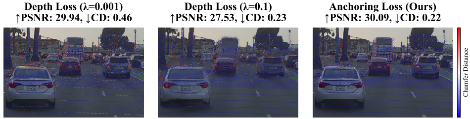
Figure 4: Depth Supervision. Prior work encodes camera and LiDAR into the same representation constrained with a LiDAR-supervised depth loss. As cross-sensor data is not fully consistent, this forces the representation to prioritize camera instead of LiDAR quality ( left ) or the inverse ( middle ), as shown by PSNR and chamfer distance. We factorize each modality into its own particle set joined via nearest-neighbor anchoring loss, improving the quality of each ( right ).
