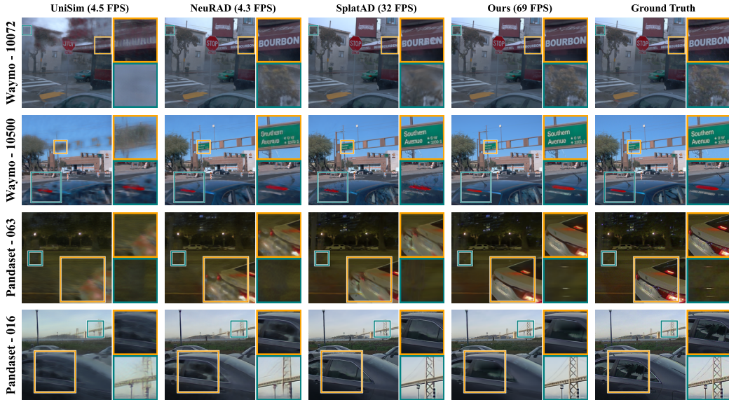
Figure 6: Dynamic Scenes. FPS numbers are averaged across Waymo Dynamic and PandaSet . Approaches that use CNNs for upsampling (Yang et al., 2023b; Tonderski et al., 2024) or view dependence (Hess et al., 2025) struggle with blurriness and incorrect lettering ( first two rows ). Our rolling shutter strategy handles rapid movement that SplatAD’s does not ( third row ). We capture background details and reflections ( bottom ) better than other methods.
