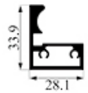
JM-6DD-04 Weight: 0.73kg/m
