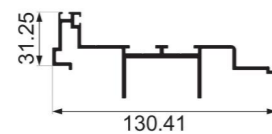
JY-120-10 outframe closing Weight : 1.652 kg/m
