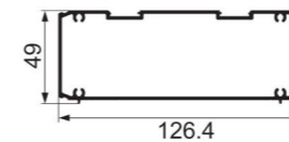
JNW-XT863 intelligent two-rail top rail Weight : 1.63 kg/m
