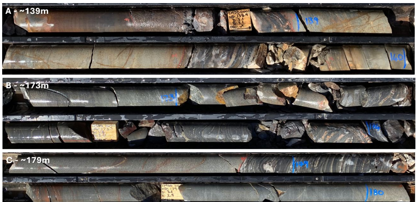
Figure 7. Diamond core photographs of the iron-rich sediments of the Dead Bullock Formation (DBF). A) At approximately 139m, folded iron-rich sediments of the DBF. B) Folded siltstone and shale units of the DBF at ~173m, with multiple folding and shearing events overprinted, with k-feldspar alteration. C) Sediments of the DBF, with increased pyrite and quartz veining.
