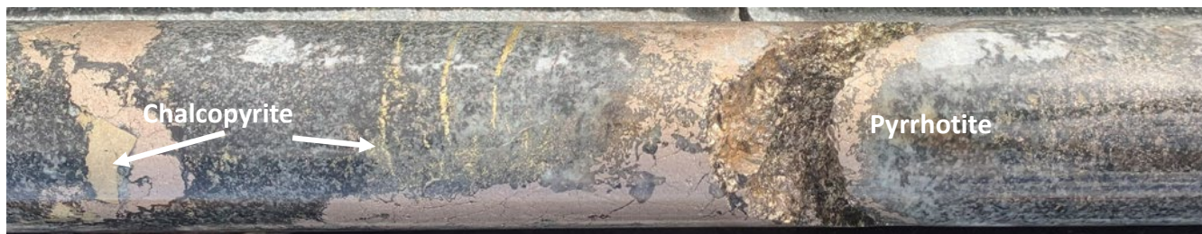
Figure 8. Massive sulphides in TMDD0001, chalcopyrite, pyrrhotite and pyrite observed, 841m depth.
