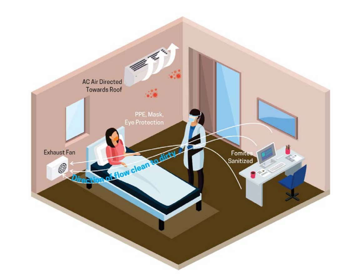
Supplementary Fig. 1 Minimising risk of transmission- All wear masks, HCW with goggles-PPE, Exhaust ventilation-aerosols exhausted, droplets on various surfaces and AC directed from clean to contaminated.
