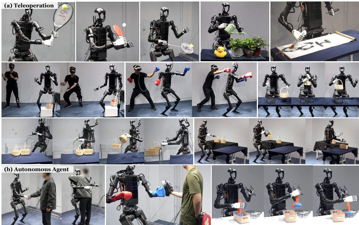
Figure 9.1. (a) OmniH2O enables teleoperating a full-size humanoid robot (Unitree H1) to complete tasks that require both high-precision manipulation and locomotion. (b) OmniH2O also enables full autonomy through visual input, controlled by GPT-4o or a policy learned from teleoperated demonstrations. Videos: see the anonymous website https://anonymous-omni-h2o.github.io/
