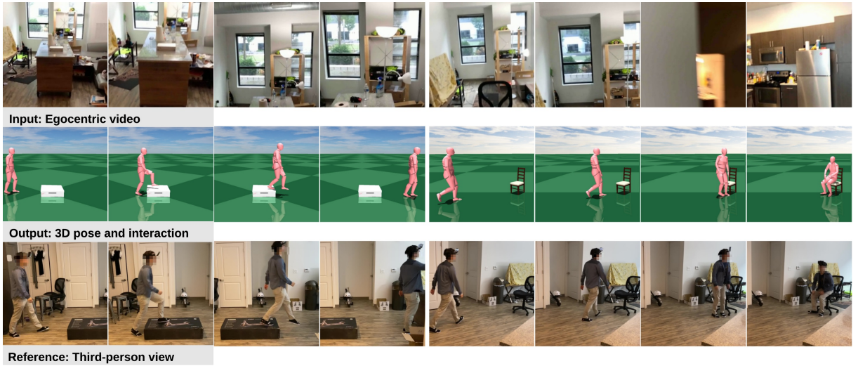
Figure 2.1. From egocentric videos, we infer physically-plausible 3D human pose and human-object interaction.
