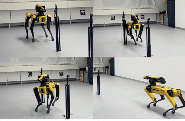
Fig. 5: Spot open-loop zig-zag trajectory obtained through trajectory optimization with the learned model.
