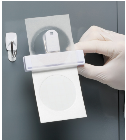
Figure 2. Example of air sampling using Neogen® Petrifilm® Plates
