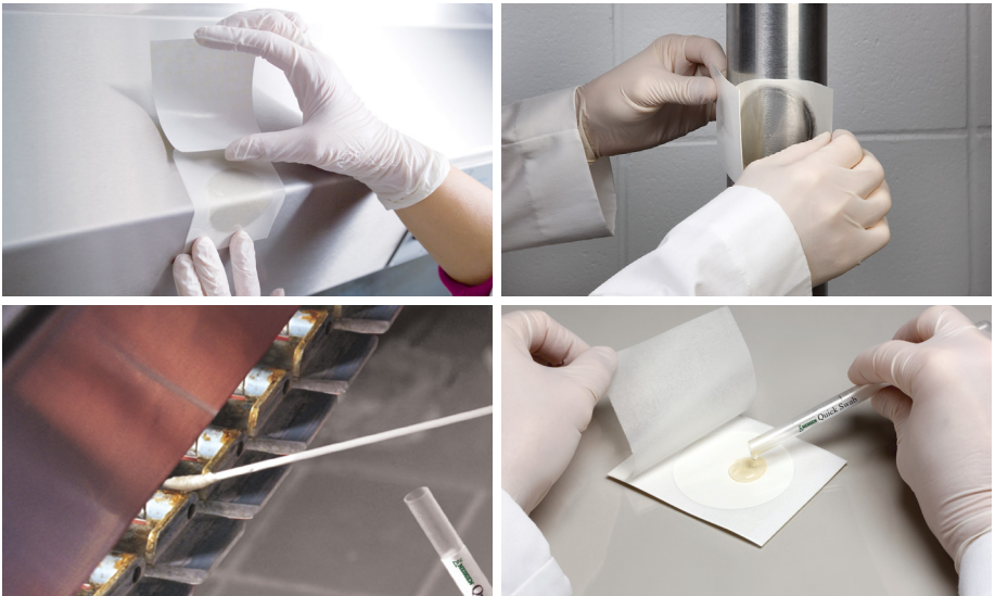
Figure 1. Examples of direct contact and swab sampling using Neogen® Petrifilm® Plates
