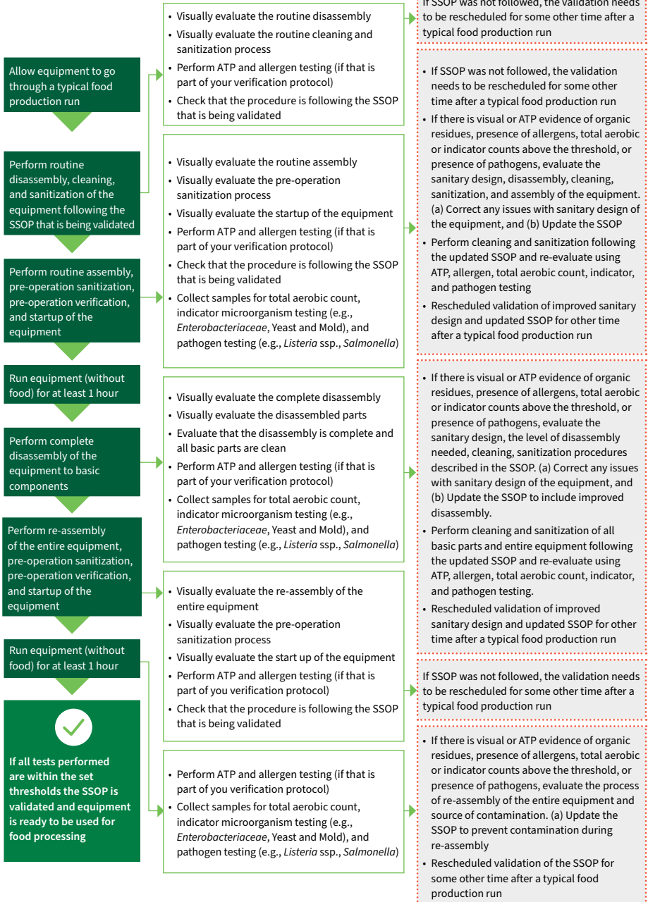
Figure 3. General workflow for validation of non-process controls and pre-requisite programs aligned within an environmental monitoring program; interpretation of results and next steps
