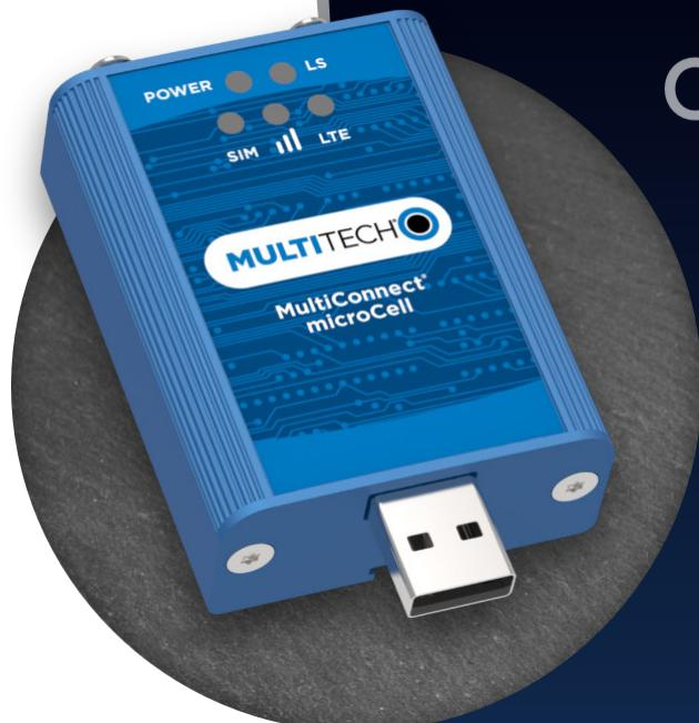
MultiConnect® microCell is a compact and simple communications platform that makes adding private LTE connectivity to existing assets quick and easy. Intended for use in settings such as vending, control systems, digital signage, smart parking, smart inventory, audio devices, notebooks and tablets.
