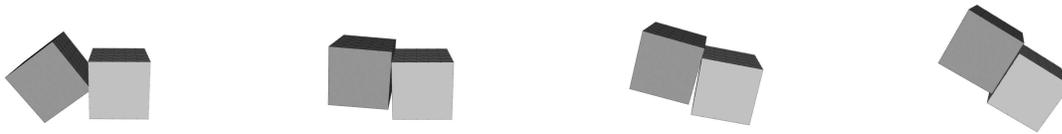
Figure 7.32: A sequence in a first-order world simulation where two objects of different mass are aligned. The left box has less mass than the right box. The left box is pulled to the right. Observe that the heavier box on the right is less affected than light box on the left in comparison with Figure 7.31.
