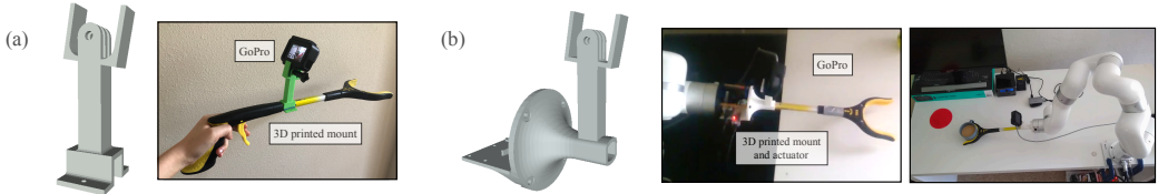
Figure 7: In part (a), we show the setup for collecting human demonstrations. This includes a 3D printed mount, a camera, and the reacher-grabber stick. Part (b) displays the corresponding setup on the robot.
