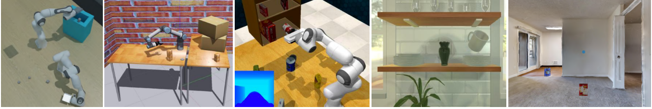
Figure 6. Suite of experimental testbeds. We contribute a set of experimental testbeds for rearrangement, spanning a spectrum of environment complexities, and agent navigation and manipulation capabilities. From left to right: T1: bimanual sweeping, T2: table organization, T3: storing groceries, T4: room rearrangement, T5: house cleanup.
