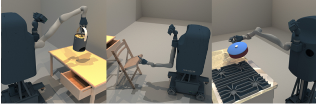
Figure 4. Full physical simulation. A simulated robot interacting with the environment in the SAPIEN [76] framework. Full physical simulation provides the highest fidelity in terms of modeling object interaction, but also a more challenging setting necessitating continuous feedback control.
