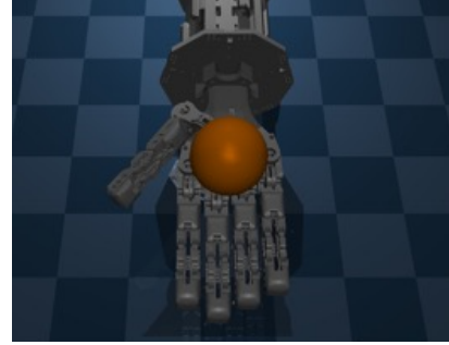
Fig. 6: CRAFT in MuJoCo Simulation. CRAFT grasping a sphere, with rolling contact joints modeled as equality constraints and joints treated as revolute constraints.
