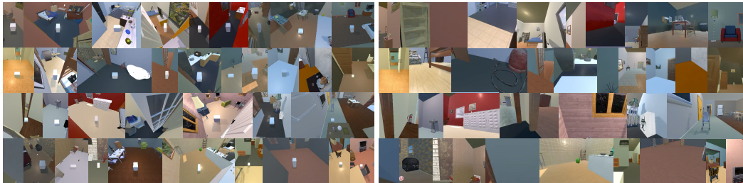
Figure 13: Random embodiments in the AI2-THOR simulator. Right column shows the egocentric view from the main camera and the left column shows a third-person view of the agent –white boxes indicate the robot colliders for visualization purposes only.
