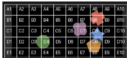
Figure 7: The Region-Based Placement Tool overlays the workspace with a labeled grid, allowing the VLM to reference specific spatial locations when issuing placement commands.
