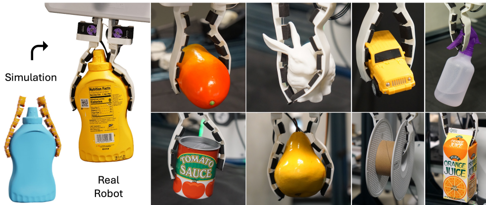
Figure 1: We introduce a co-design framework that jointly optimizes the spatial stiffness distribution and grasping poses of soft grippers via a simulation-trained neural surrogate. Hardware experiments demonstrate that our optimized grippers outperform both rigid and overly compliant designs.
