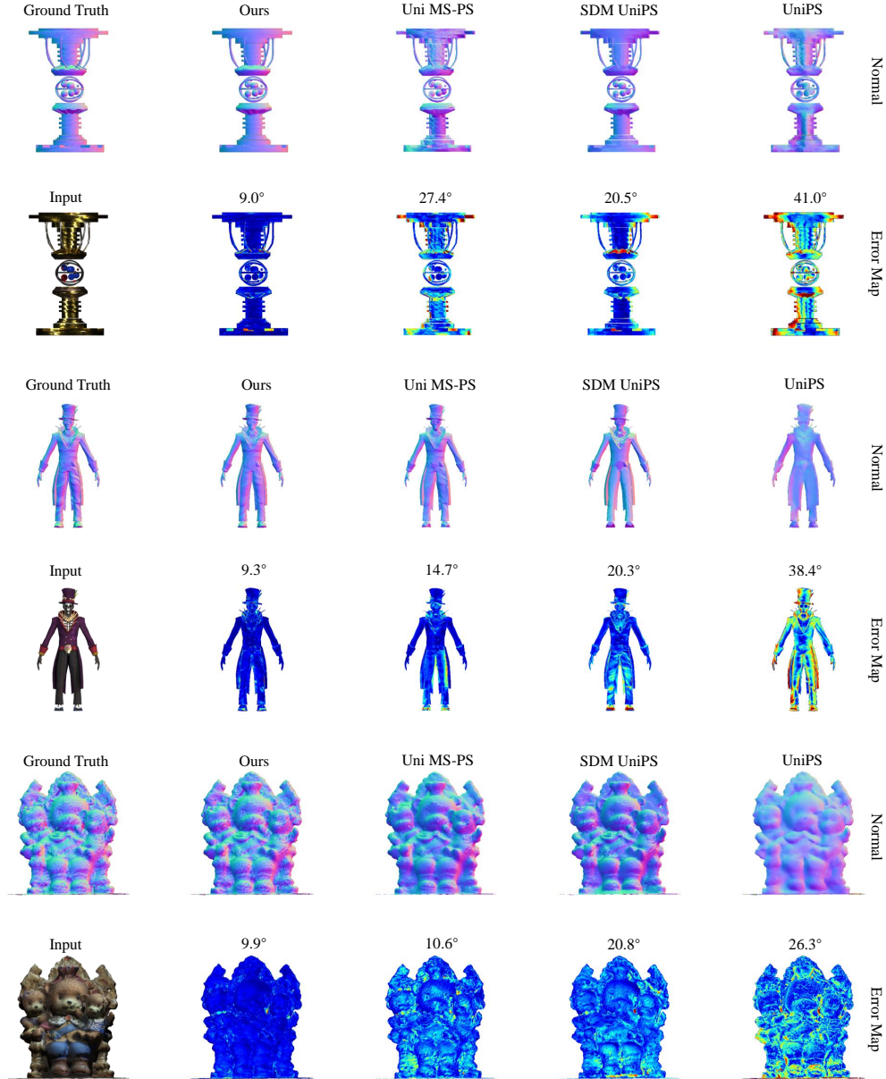
Figure A13: Comparison of different Universal PS methods on our PS-Verse Testdata, showcasing ground truth normals, reconstruction normals, and corresponding error maps. The error maps depict the Mean Angular Error (MAE), measured in degrees; lower MAE values signify a more accurate reconstruction.
