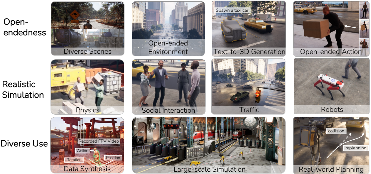
Figure 1: An Overview of the SIMWORLD Simulator , featuring three key designs: (1) realistic, open-ended world simulation, (2) rich interface for LLM/VLM agents, and (3) diverse physical and social reasoning scenarios.
