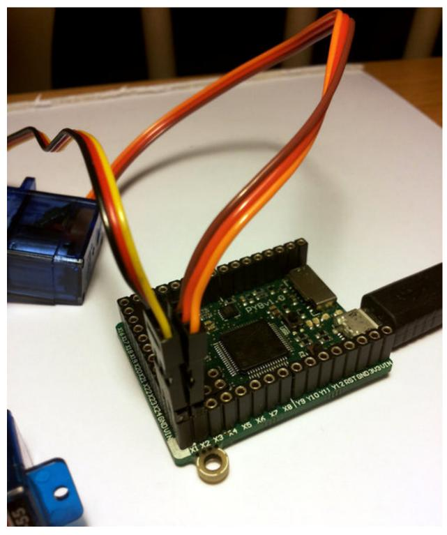
In this picture there are male-male double adaptors to connect the servos to the header pins on the pyboard.
