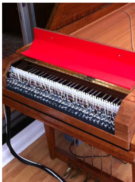
The U.A.V. with lid opened so that the solenoids can be seen moving.
