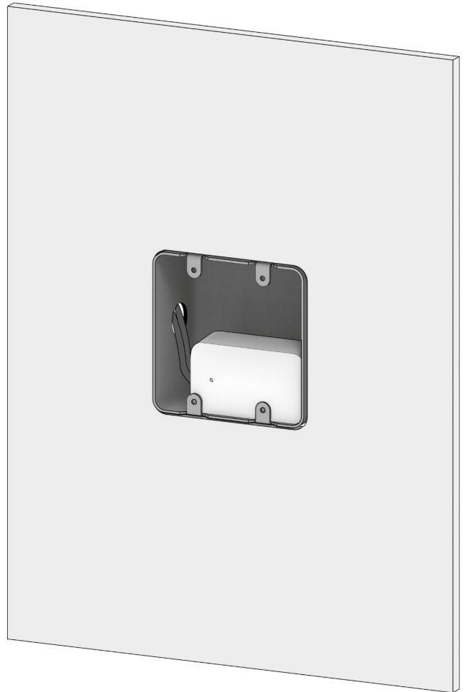
Placing inside a junction box
