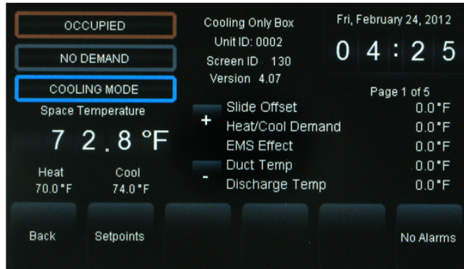
Figure 37: VAV/Zone Controller Status Screen
