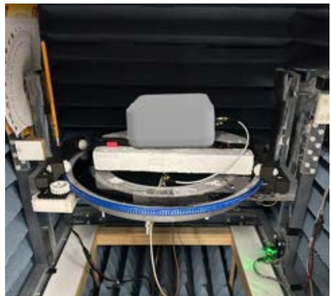
Fig. 2-2 Generic IoT Device placement in chamber
