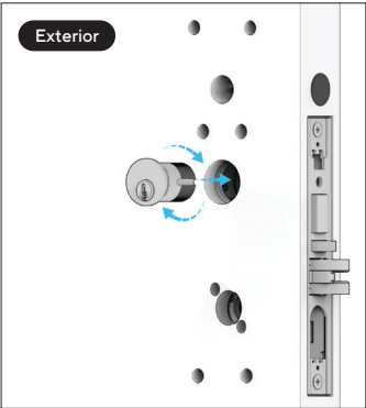
Insert the Key Cylinder and turn it clockwise into the Cassette.
