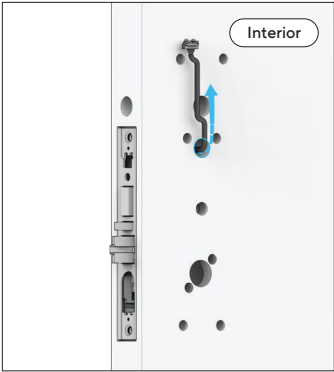
Route the Cassette Cable through the lock cable hole on the interior side.
