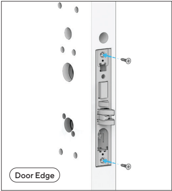
Use the Cassette Mounting Screws from the Screw Holder, in the Install Kit, to fasten the Cassette.
