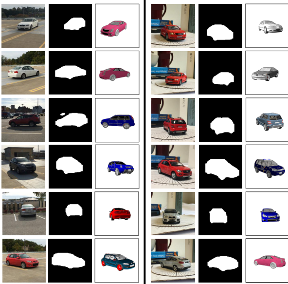
Figure 7: Some of the initialization results on natural sequences are shown in this figure. Results on real cars in the wild are shown on the left while results on toy model cars are shown on the right. Each row contains a combination of RGB image of first frame, silhouette of first frame, template retrieved from our style & pose initialization. Despite color, the retrieved model are close in shape and appearance.
