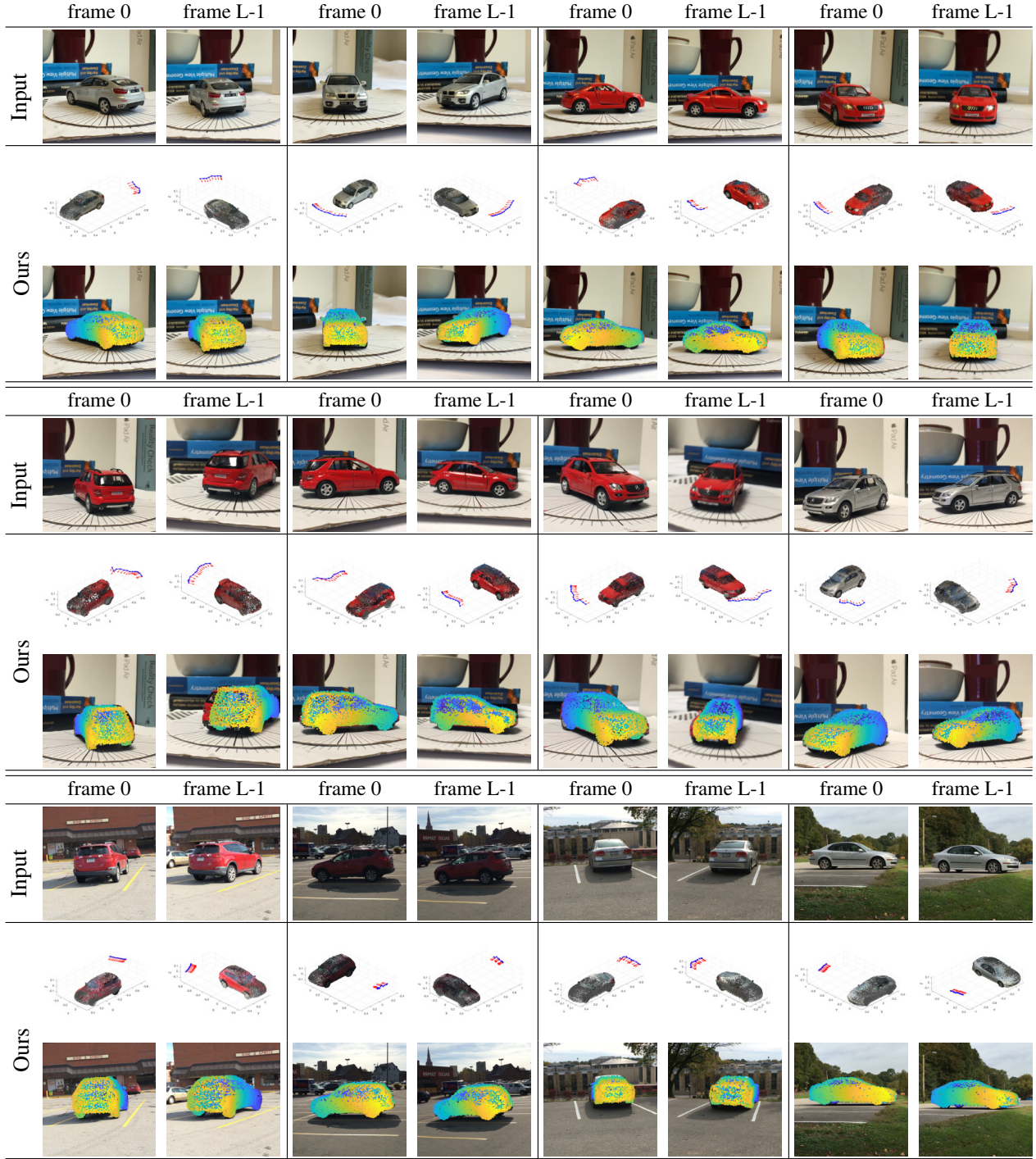
Figure 2: More results on natural sequences. For each sample sequence, we show the first and last frame of the sequence (first row), the recovered shape and camera poses in two views (middle row) and the reprojected points onto the first and last frame, colored with the inverse depths (brighter is closer). For the recovered shape, we color the visible points with pixel values from the frames, and the invisible points with grey.
