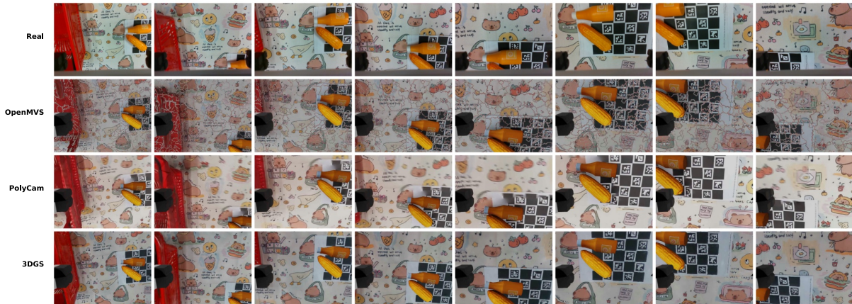
Fig. 4: Visual comparison of rendering approaches. Rendering results of reconstruction outputs from PolyCam, OpenMVS, and 3DGS, compared with real-world photos.
